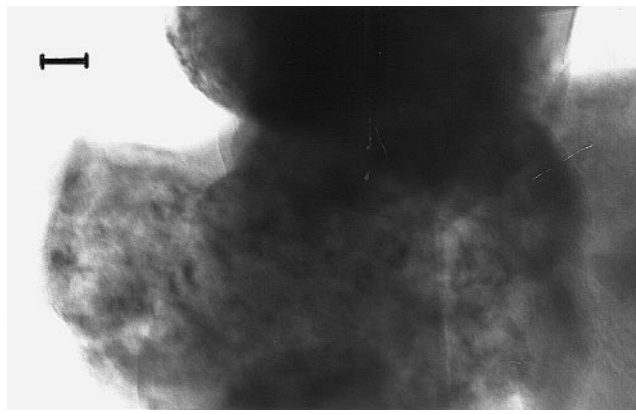
FIG. 6. TEM pattern (bar = 10 nm) for \text{LaMn}_{1-x}\text{Cu}_x\text{O}_3 with x = 0.6 calcined at 1073 K.
